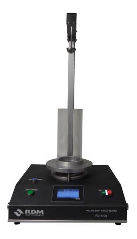
The FD-1709 is a cost effective solution for testing impact resistance of sheet materials. Bench mounted or floor standing, with drop heights and darts for ASTM D1709 Methods A & B. Operation is by push button, and an optional touchscreen provides a standard operating procedure and test traceability.
